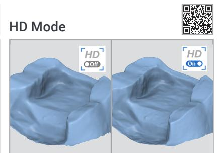
Get a sharper scan image in the margin area with the upgraded HD Mode.
