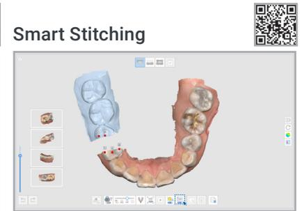
Scan with your own scanning strategy. Fragmented scan data are aligned with automatically detected common area.
